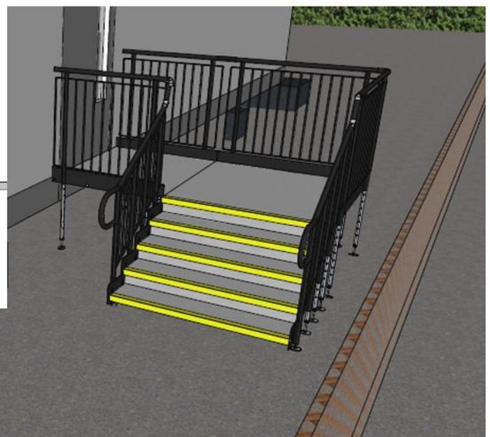
**END RESULT:** A steel rental ramp and two sets of step units were installed. These will be on hire until the work on the permanent main building is finished.
