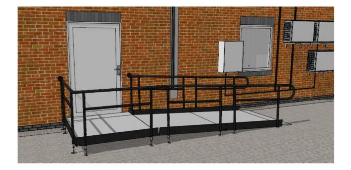
**END RESULT:** A emergency exit ramp with a 1:15 gradient was installed, after the new door had been fitted.
