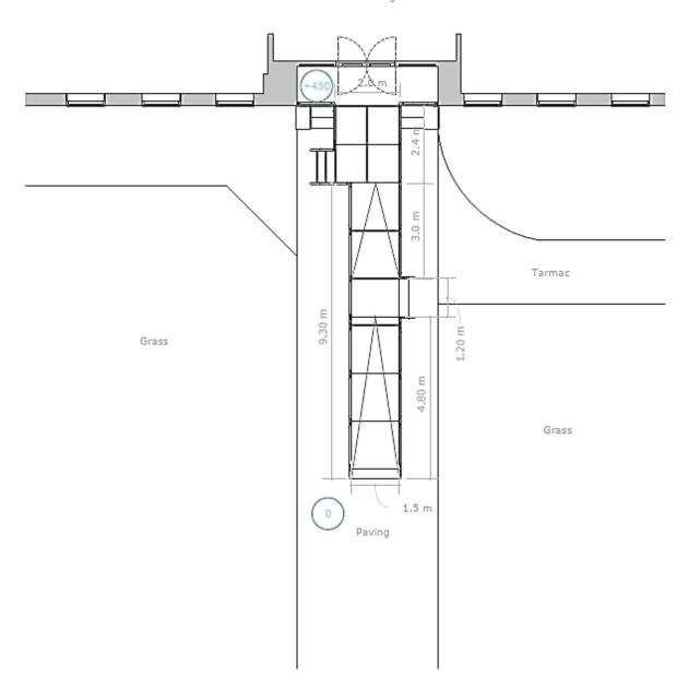
**END RESULT:** Our team installed a Rapid Ramp with a 1:15 gradient. It included two steps units and self-draining platforms.
