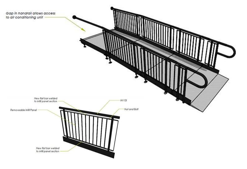
**END RESULT:** The Rapid Ramp includes a 1:15 gradient and fully complies with documents M & K of the building regulations.
