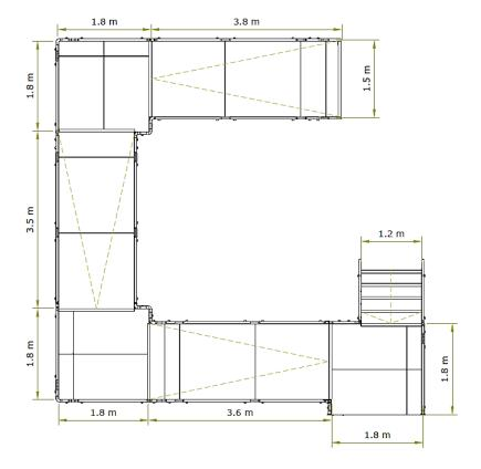
**END RESULT:** The system was installed over concrete and took only two days to complete. Plus, it includes a compliant 1:15 gradient.
