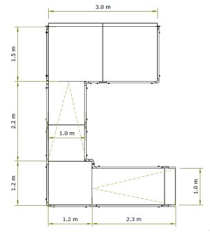
**END RESULT**: Once the new door was fitted, the ramp was Installed in a horseshoe shape configuration within a day, minimizing disruption.
