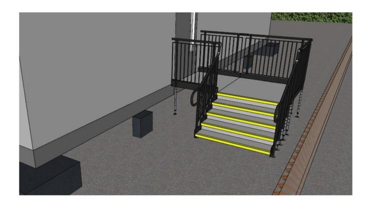
**END RESULT:** A rental ramp and two sets of step units were installed. These will be on hire until works on the permanent main building is finished.
