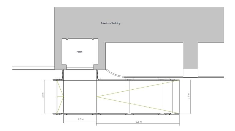
**END RESULT:** Once the old concrete ramp had been broken up, we installed a modular Rapid Ramp within a morning. This prevented the installation encroaching on the afternoon hall bookings.
