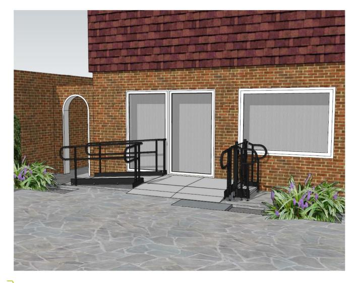
**END RESULT:** A two metre wide access platform was included to provide manoeuvring space for the wheelchair. Plus, it took only a few hours to install and was immediately functional.
