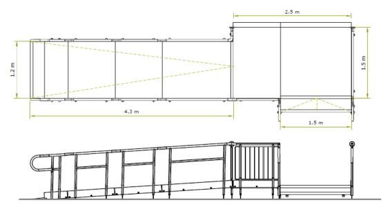
END RESULT: A modular ramp with a 1:15 gradient was installed with a few hours.
