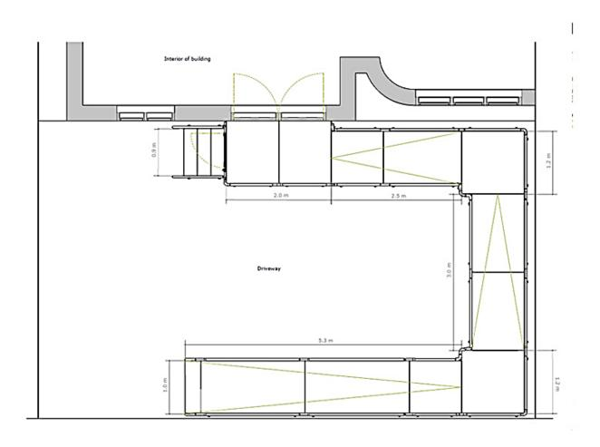
**END RESULT:** A ramp with a 1:12 gradient was installed with a few hours. It included adjustable access steps for able-bodied users.
