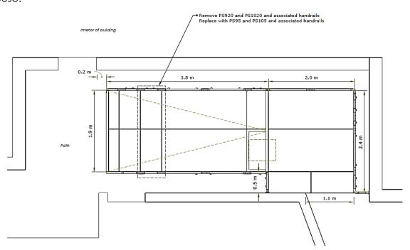
**END RESULT:** A fully compliant ramp with a 1:15 gradient was installed with a few hours.
